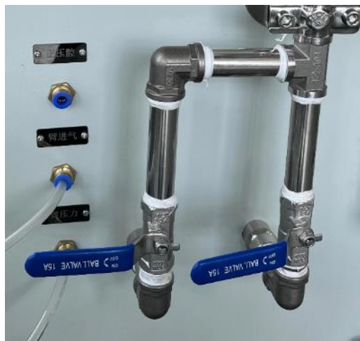
Figure 15 Closed state of the explosion-proof cabinet air inlet valve
