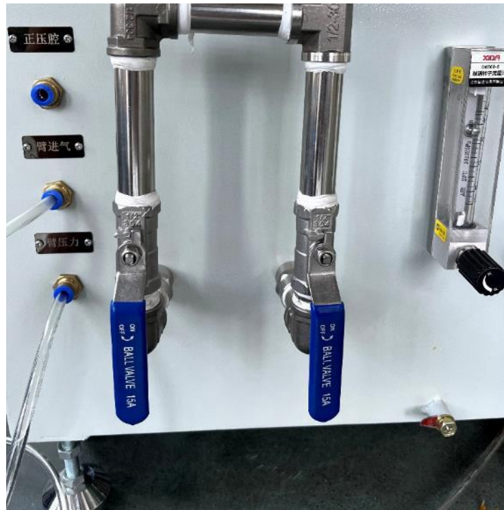
Figure 20 Air inlet valves of the robotic arm and explosion-proof cabinet are in open state
