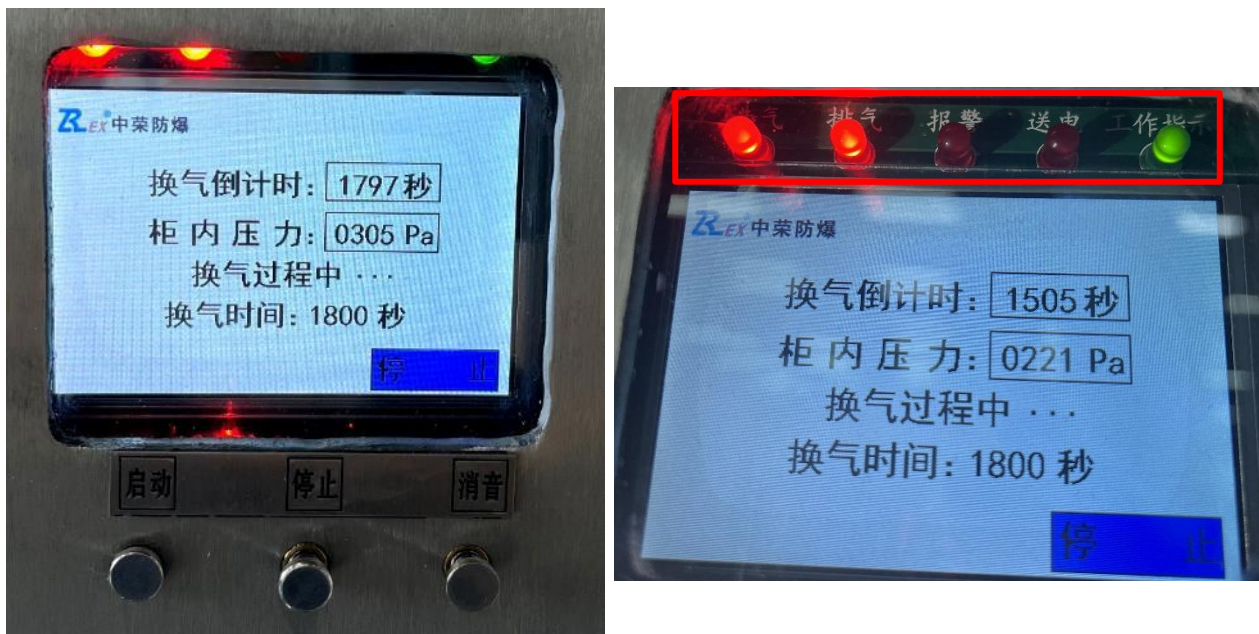
Figure 23 Ventilation state and display lamp state
