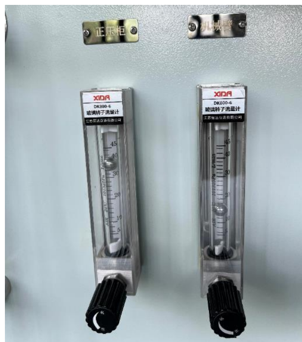
Figure 21 Air intake flows of the robotic arm and explosion-proof cabinet
