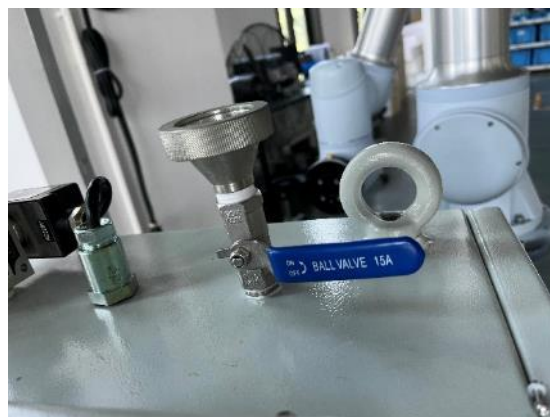
Figure 16 Closed state of the exhaust valve at the top of explosion-proof cabinet
