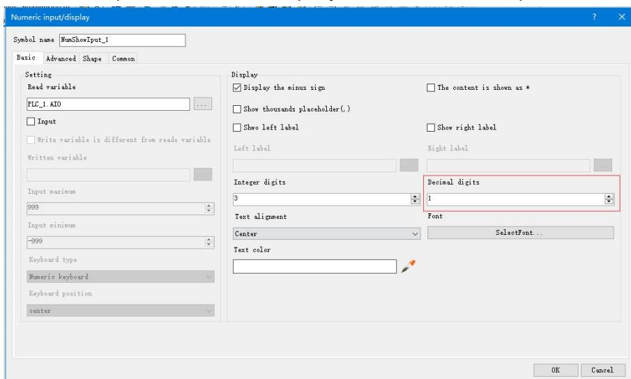
So that when the PLC read AI0 value, AI0=123, that is the actual value of 12.3°C, there is no need to have data processing in PLC and configuration, only set the 1 decimal places on the numerical display primitive, then it will be automatically reduced by 10 times, displaying value of 12.3, that is the actual value of 12.3°C.
