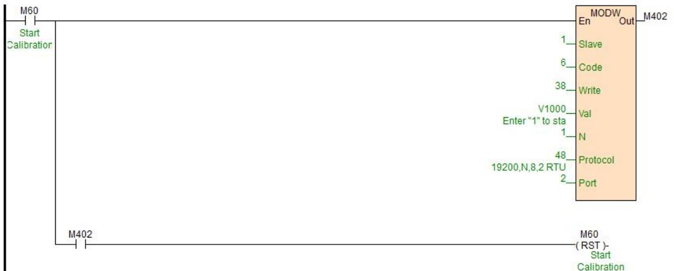
//Network 3 Step3: In the first segment of calibration, put a standard weight on the pan connected to the load cell module. The weight of the counterweight should be written into CR27H(16 bits) You could continue to step 6 if multiple segments of calibration are unnecessary.
