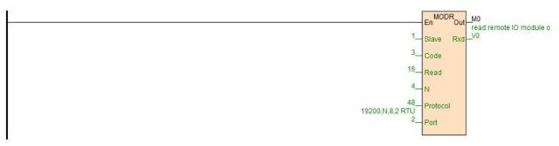
The host PLC reads the 4-channel temperature values of TE-4RC by Modbus read instruction MODR, the start address is 10H (hexadecimal), that is, the decimal value is 16. When the communication is successful, M0 is ON, the temperature values which are read back will be stored in V0-3, V0=235, indicating that the actual temperature of the first channel is  $23.5^{\circ}$ C, the same as V3=867, indicating that the actual temperature of the fourth channel is  $86.7^{\circ}$ C.
