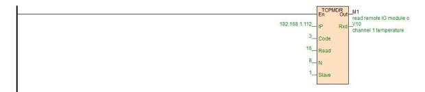
1.8 Remote IO appliciation example: HTCloud Designer configuration communicates directly with TE-8TC module
